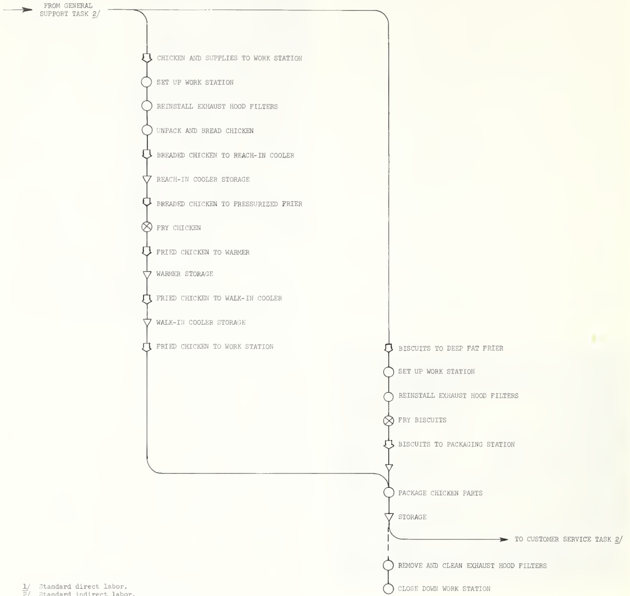
Figure 19.—Flow process chart for chicken parts.
